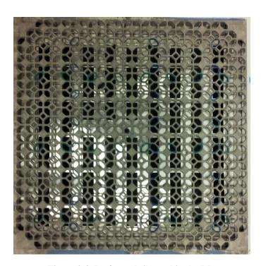
Figure 2.4: Perforated tile used in the RL.
