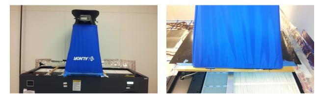
Figure 3.2: Backflow measurements on top of CRAH-2 via TSI Flow Hood.
